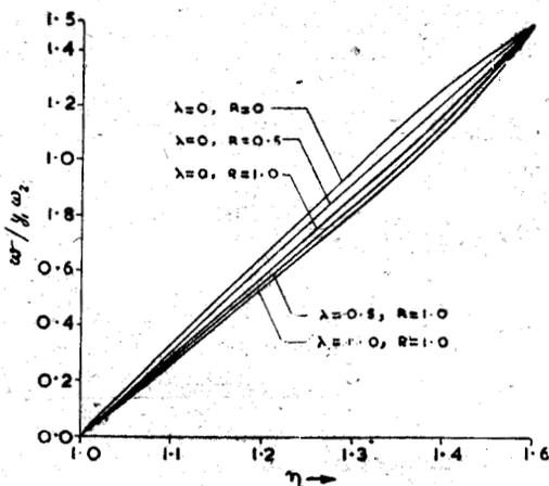
Fig 2—Shearing stress at the inner cylinder  $\tau/\mu\omega_2$  vs  $R$  when the inner cylinder is at rest for various values of  $\lambda$ .
