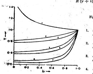
Fig. 2—Temperature distribution behind the shock wave, thin case, j=1
