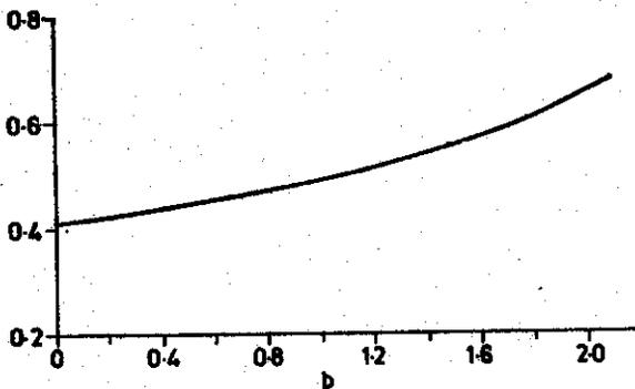
Figure 4. Time required to reach steady state vs rate of heat generation.
