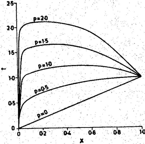
Figure 1. Steady state temperature for different rates of heat generation.
