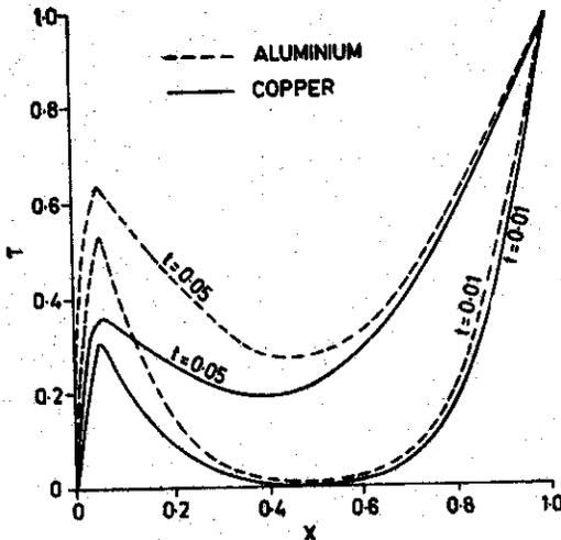
Figure 3. Comparison of temperature distribution in aluminium and copper for different times.
