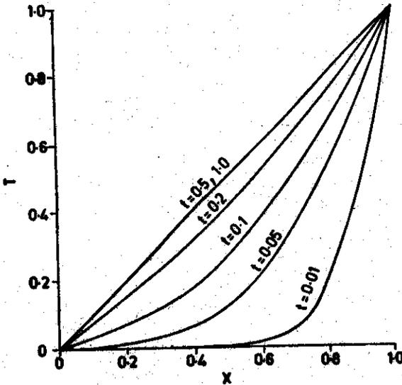
Figure 5. Time history of temperature in the slab without heat sources.
