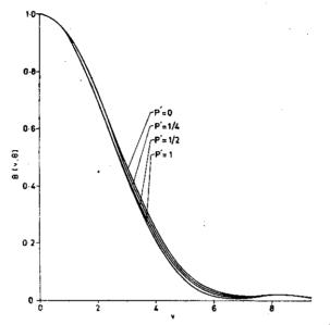
Figure 2. Intensity distribution at  $\theta = \pi/4$  for different degrees of polarisation P' in case of EPL beam in which  $\epsilon' = \pm \pi/6$  and  $\theta' = 0.0$ .
