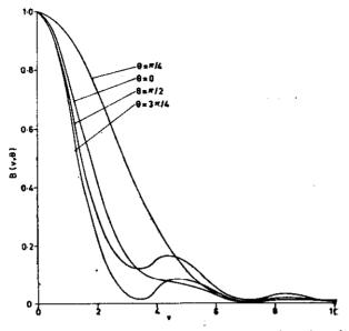
Figure 5. Intensity distribution for different orientation of analyser  $\theta$  in case of EPL beam in which P' = 1.0,  $\epsilon' = \pm \pi'/6$  and  $\theta' = \pi/4$ .
