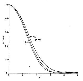
Figure 4. Intensity distribution at  $\theta = \pi/4$  for different values of azimuth  $\theta'$  in case of EPL in which P' = 1.0 and  $\epsilon' = \pm \pi/6$ .
