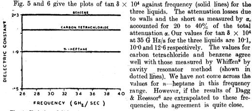
Fig. 4-Variation of dielectric constant with frequency for three low loss liquids.
