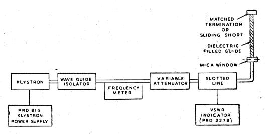
Fig. 3-Block diagram of the experimental setup.
