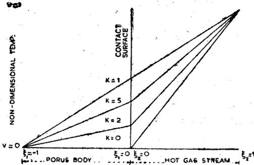
Fig. 2—Temperature distribution for different conductivity ratio  $K$  when Eckert number  $E_g = 0$  and injection is absent.
