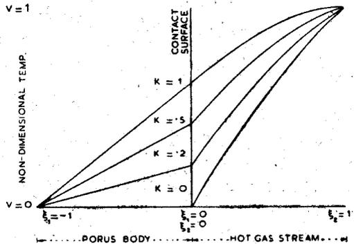
Fig. 3—Temperature distribution for different conductivity ratio  $K$  when Eckert number  $E_g = 1$  and injection is absent.
