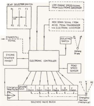
Figure 4. Automatic transmission controller of heavy vehicle.
