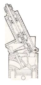
Figure 3(b). Helenoid valve actuator.
