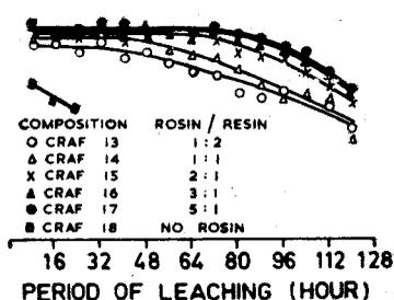
Figure 3. Leaching rate characteristics of antifouling paints with cuprous oxide PVC of 43% and different rosin to resin ratio. (Accelerated leaching rate  $\mu\text{g}$  of  $\text{Cu}/\text{cm}^2/\text{day}$ )
