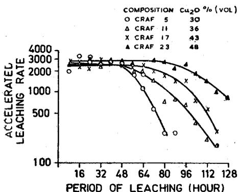
Figure 2. Leaching rate characteristics of antifouling paints with rosin to resin ratio of 5:1 and different PVC of cuprous oxide. (Accelerated leaching rate  $\mu\text{g}$  of  $\text{Cu}/\text{cm}^2/\text{day}$ )
