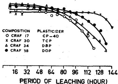
Figure 5. Leaching rate characteristics of antifouling paints containing different plasticizers in presence of rosin. (Accelerated leaching rate  $\mu\text{g}$  of  $\text{Cu}/\text{cm}^2/\text{day}$ )
