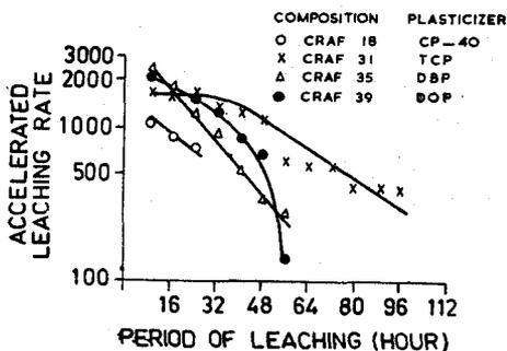
Figure 4. Leaching behaviour of rosin free antifouling paints containing different plasticizers. (Accelerated leaching rate  $\mu\text{g}$  of  $\text{Cu}/\text{cm}^2/\text{day}$ )
