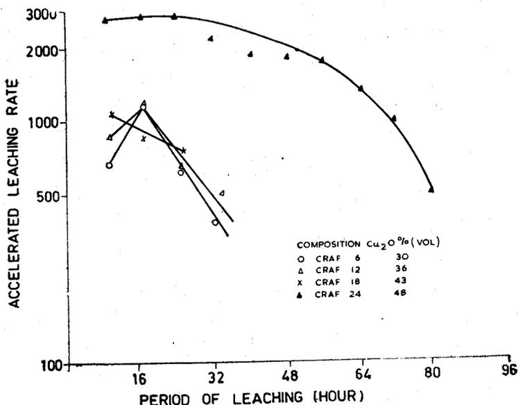
Figure 1. Leaching behaviour of rosin free antifouling paints containing different amount of cuprous oxide and Chlorinated paraffin wax. (Accelerated leaching rate  $\mu\text{g}$  of  $\text{Cu}/\text{cm}^2/\text{day}$ )
