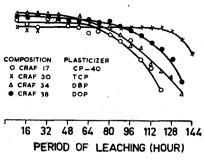
Figure 5. Leaching rate characteristics of antifouling paints containing different plasticizers in presence of rosin. (Accelerated leaching rate  $\mu g$  of Cu/cm<sup>2</sup>/day)
