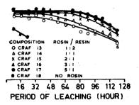
Figure 3. Leaching rate characteristics of antifouling paints with cuprous oxide PVC of 43%and different rosin to resin ratio. (Accelerated leaching rate  $\mu g$  of Cu/cm<sup>2</sup>/day)
