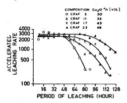
Figure 2. Leaching rate characteristics of antifouling paints with rosin to resin ratio of 5:1 and different PVC of cuprous oxide. (Accelerated leaching rate  $\mu g$  of Cu/cm<sup>2</sup>/day)
