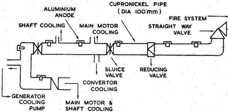
Figure 8. A schematic view of a small *Kunifer-5* pipe section fitted with aluminium alloy anodes.
