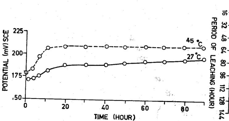
Figure 5. Potential time decay behaviour of *Kunifer-5* alloy in seawater at 27°C & 45°C.
