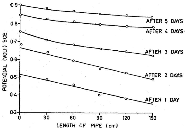
Figure 7. Variation of potential along the length of cathodically protected tube in stagnant seawater.
