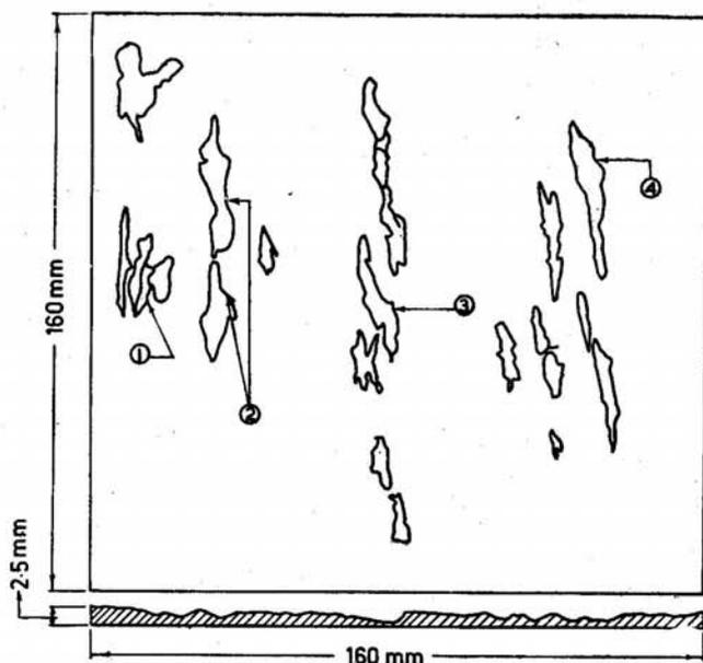
Figure 2. A sketch showing a pattern of corrosion-erosion observed on the failed *Kunifer-5* pipe 1.
