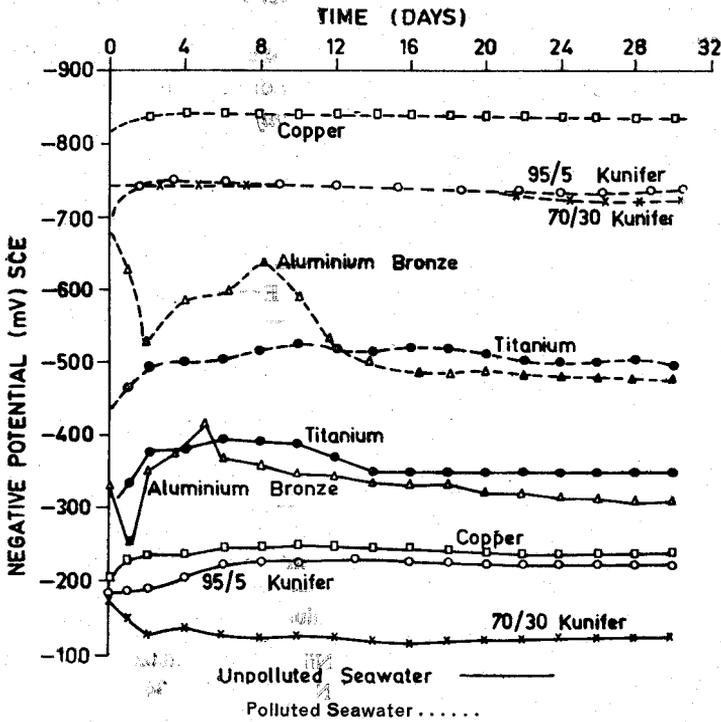
Figure 4. Potential/time decay behaviour of various copper alloys exposed to unpolluted and polluted seawater.
