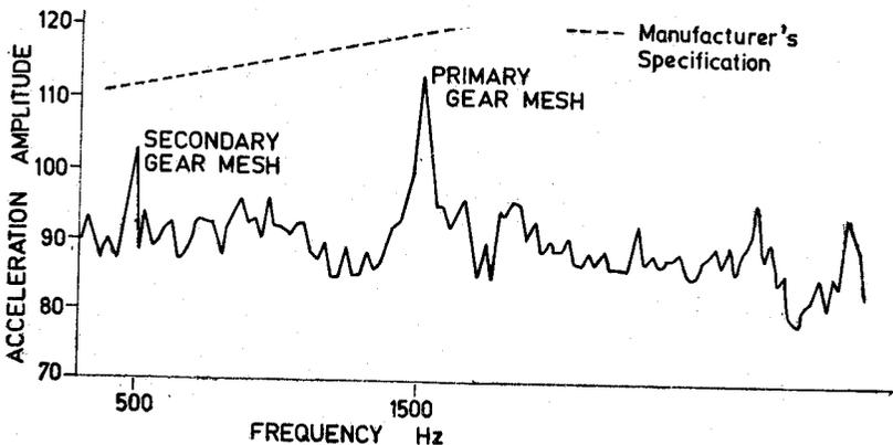
Figure 3. Narrow band analysis of gearbox vibration signature.
