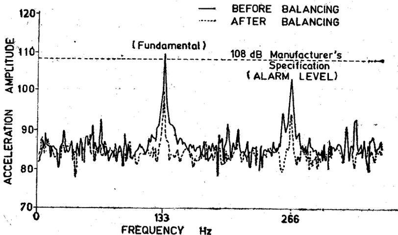
Figure 2. Narrow band analysis of steam turbine vibration signature.
