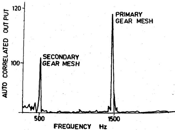
Figure 3(a). Auto spectrum analysis of gearbox vibration signature.
