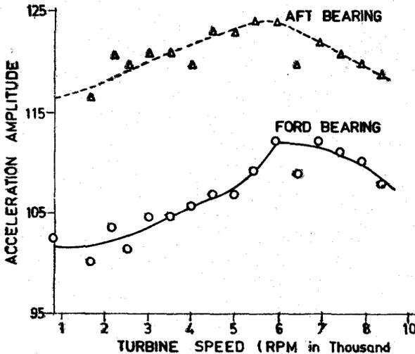
Figure 4. Turbine blade vibration amplitude variation. (Observed value 1.4 kHz, Theoretical value 1.65 KHz)
