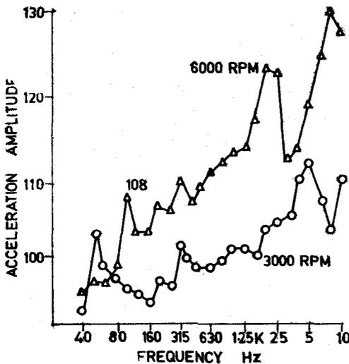
Figure 5. Vibration signature of steam turbine.
