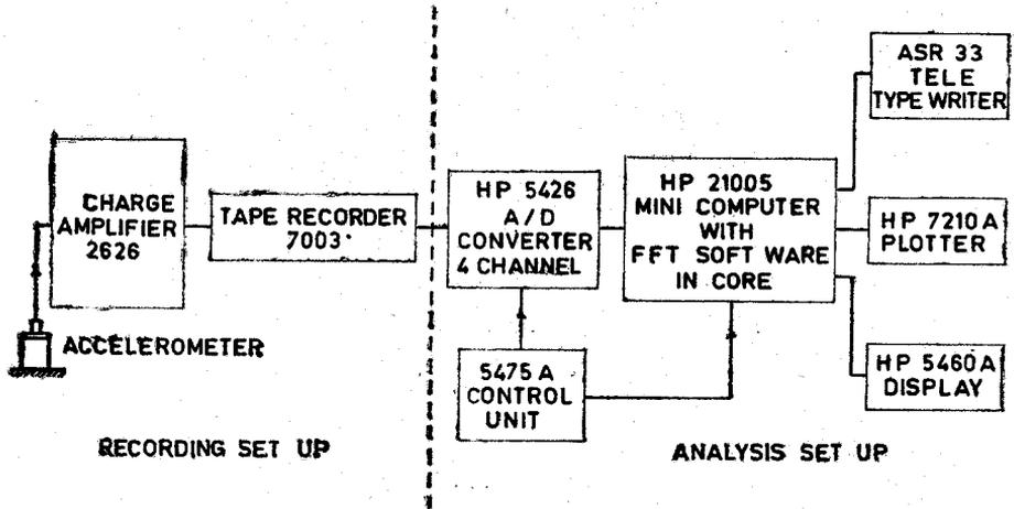
Figure 1. Vibration monitoring set up.
