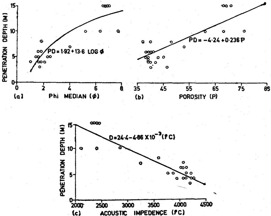
Figure 5. Regression analysis; (a) Phimedian vs penetration depth; (b) Porosity vs penetration depth; and (c) Acoustic impedance vs penetration depth.
