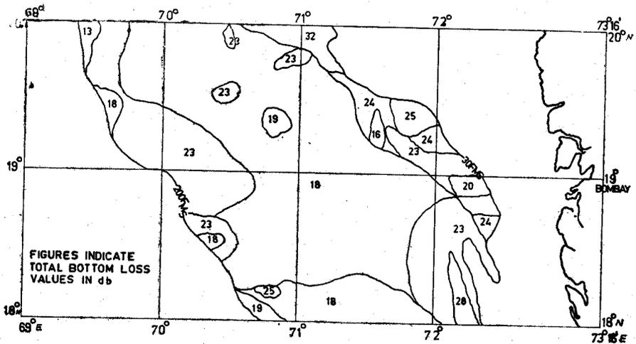
Figure 3. Bottom loss model (estimates based on 3° beam width, 7.5 KHz signal frequency at vertical incidence).
