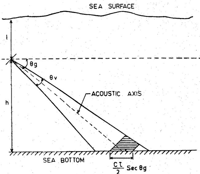
Figure 3. Geometry of the reverberation experiment.
