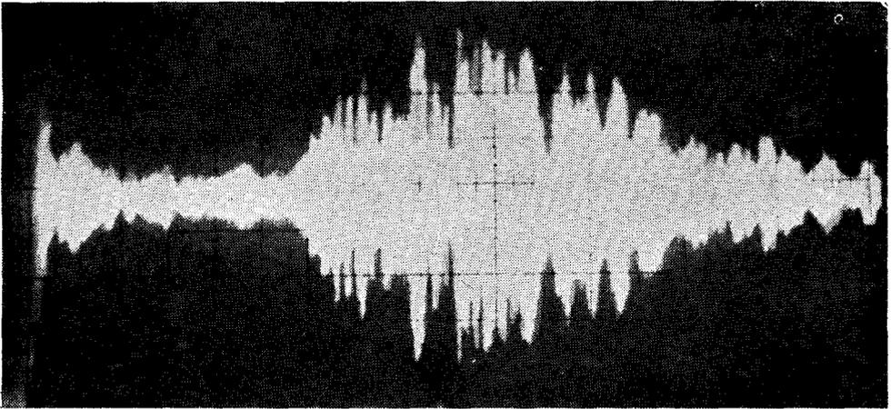
Figure 1. Reverberation returns from the rough bottom of the sea insonified by CW pulse width = 10 ms, carrier frequency  $f_0 = 9.5$  KHz.
