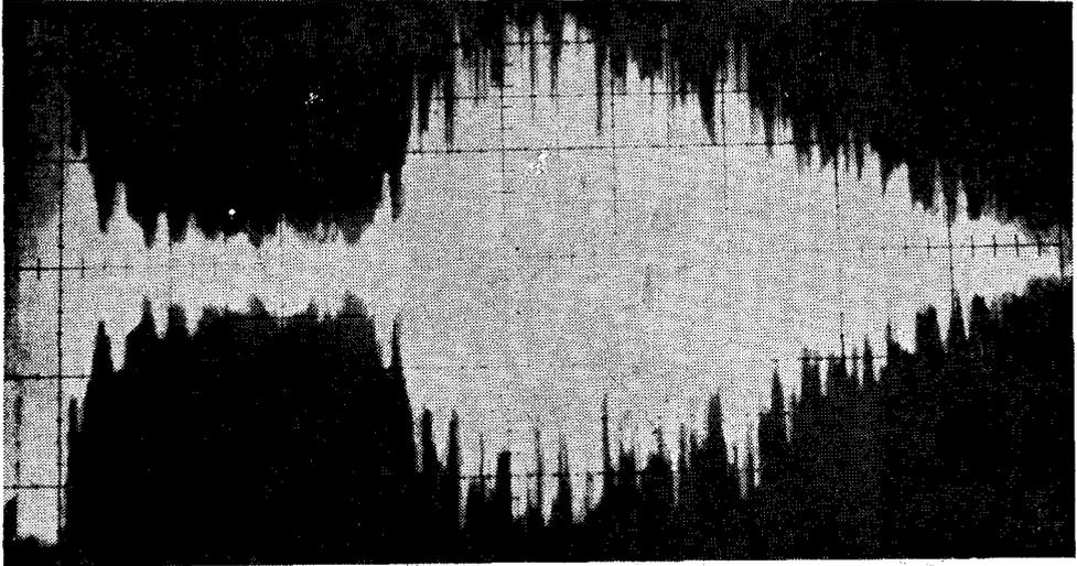
Figure 2. Reverberation returns from the rough bottom of the sea insonified by F M pulse width = 10 ms, band width = 9.3-9.7 KHz.
