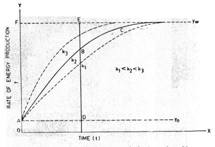
Figure 1. Theoretical relationship between y and t for three values of k (schematic).
