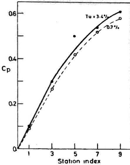
Figure 3. Pressure recovery in a straight diffuser
