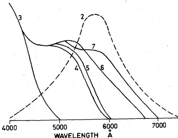
**Figure 4.** Sensitivity of different photographic emulsions over the visible spectrum (2)—Sensitivity of eye, (3)—Ordinary blue sensitive emulsion, (4)—Slow orthochromatic, (5)—Fast orthochromatic. (6)—Normal panchromatic and (7)—High speed pan emulsion with increased red sensitivity.
