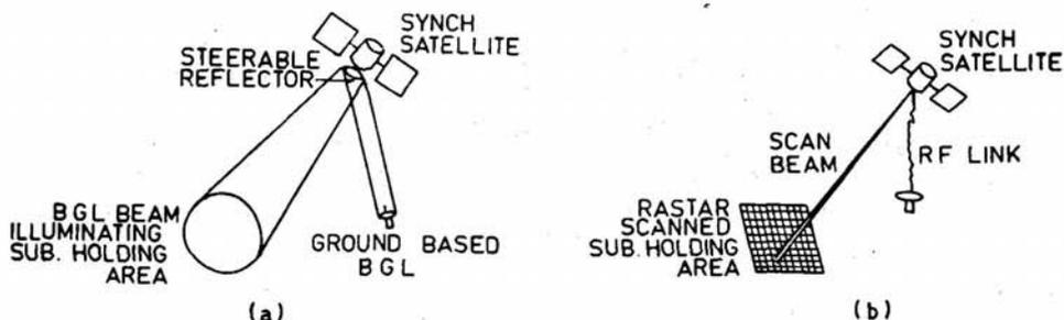
Figure 6. Two proposed schemes for satellite to submarine communication with blue green laser.
