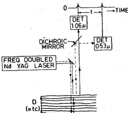
Figure 5. Schematic arrangement for sea depth profile measurement.
