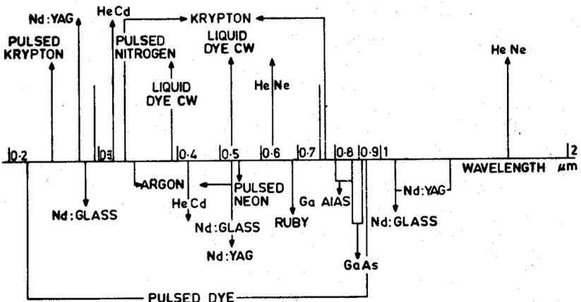
Figure 2. Spectrum of commercially available lasers in the range 0.2 – 2 $\mu$ m.
