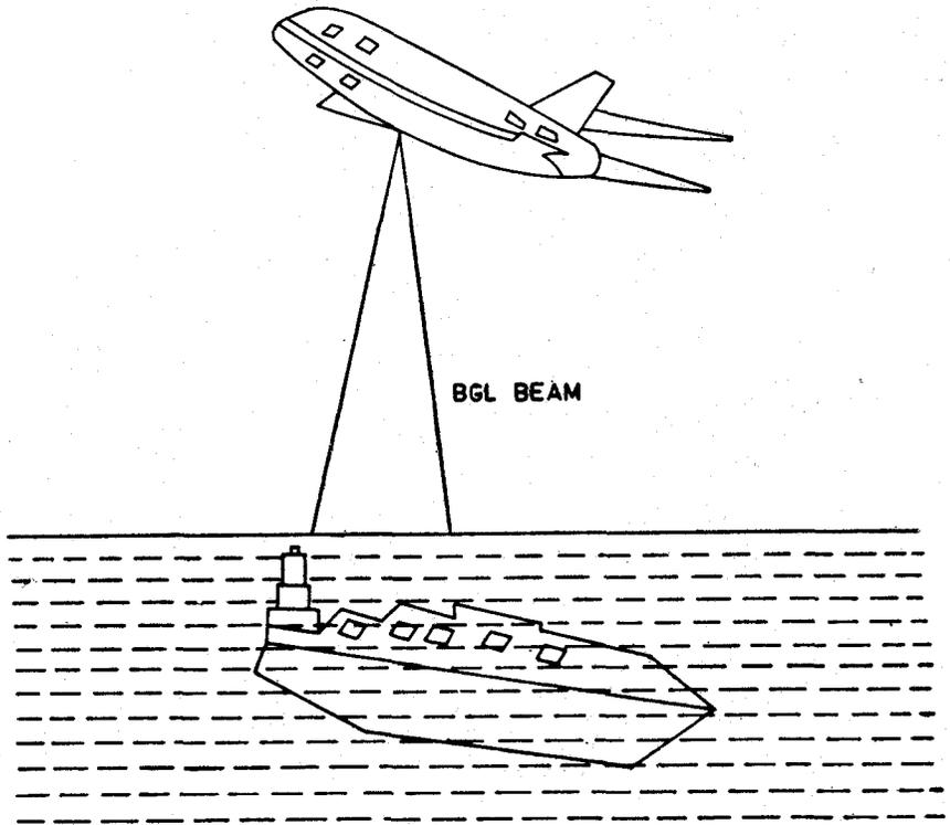
Figure 7. Aircraft mounted BGL for communication with submarine.
