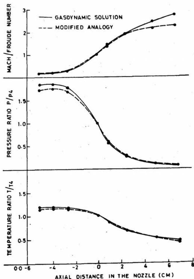
Figure 3. Comparison of mach numbers, pressure and temperature ratios, modified supersonic flow for the case in free steam velocities.
