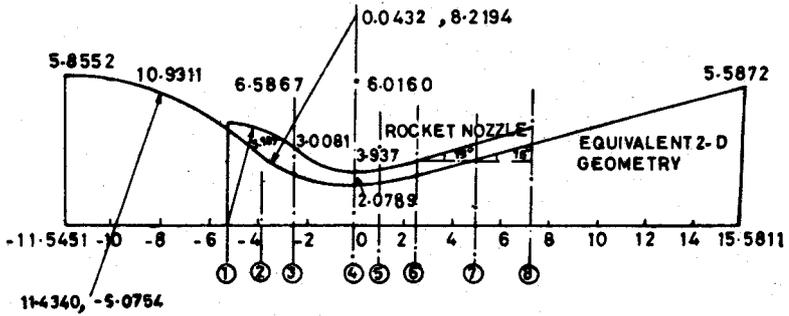
Figure 1. Axisymmetric rocket nozzle with equivalent 2-D geometry.
