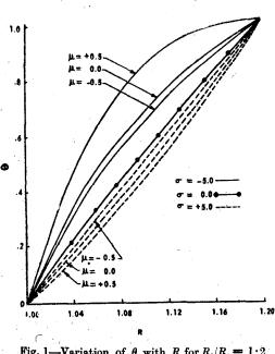
Fig. 1—Variation of  $\theta$  with R for  $R_2/R_1 = 1.2$ , E = 0.8,  $P_T = 0.9$ ,  $T_2/T_1 = 2$ ,  $R_1^3 \Omega_1/\nu$ = 600 and three different values of  $\mu$  and  $\sigma$
