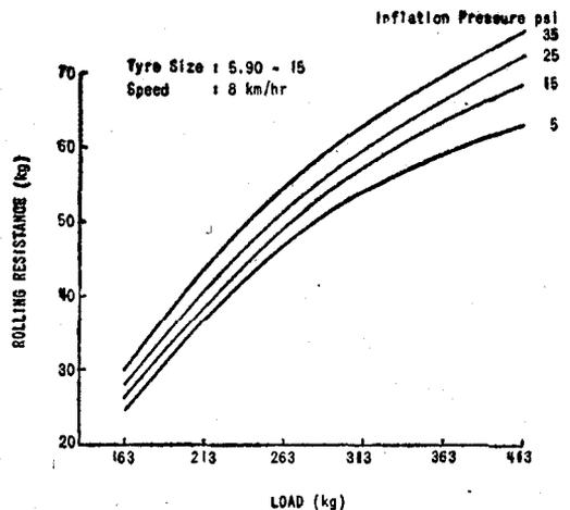
Fig. 3—Variation of rolling resistance with load at various inflation pressures for the wheel 5·90-15 at a speed of 8 kilometers per hour.
