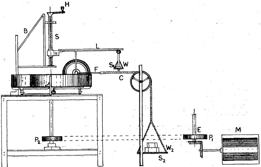
Fig. 1—Block diagram of friction apparatus for determining the rolling resistance of pneumatic rubber tyres on sand at various speeds.
