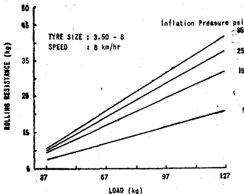
Fig. 5—Variation of rolling resistance with load at various inflation pressures for Scooter wheel 3.50-8 at a speed of 8 kilometers per hour.
