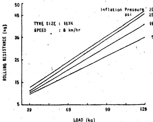
Fig. 4—Variation of rolling resistance with load at various inflation pressures for Trolley wheel 16 x 4 at a speed of 8 kilometers per hour.
