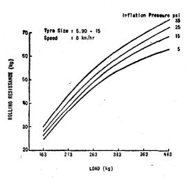
Fig. 3—Variation of rolling resistance with load at various inflation pressures for the wheel 5.90-15 at a speed of 8 kilometers per hour.
