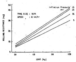
Fig. 4—Variation of rolling resistance with load at various inflation pressures for Trolley wheel  $16 \times 4$  at a speed of 8 kilometers per hour.
