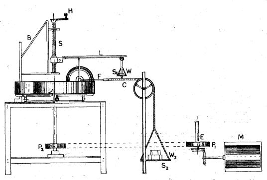
Fig. 1-Block diagram of friction apparatus for determining the rolling resistance of pneumatic rubber tyres on sand at various speeds.
