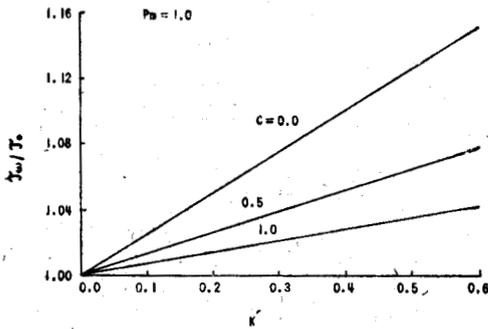
Fig. 1—Variation of skin-friction ratio against (hydromagnetic parameter)<sup>2</sup> for  $P_m = 1$ .
