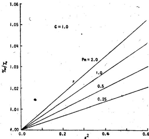
Fig. 2—Variation of skin-friction ratio against (hydromagnetic parameter)<sup>2</sup> for  $c = 1$ .
