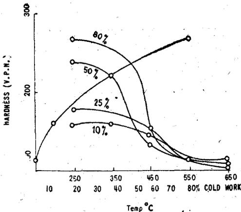
Fig. 2—Work hardening and recrystallisation of 1.06% silicon brass.
