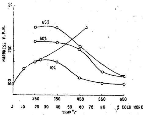
Fig. 1—Work hardening and recrystallisation characteristics of 1.86% silicon brass.
