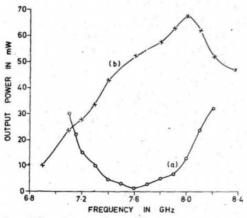
Figure 4. Power-frequency characteristics.
