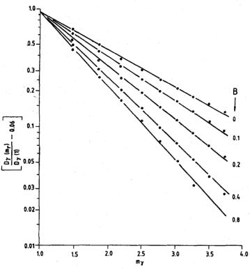
Figure 3. Relative diffuse sky radiation in relation to turbidity B and air mass  $(m_r)$ .
