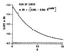
Figure 4. Exponential relationship between slope m(B) and turbidity B.
