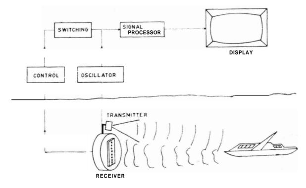
Figure 2. Holographic search system for divers.
