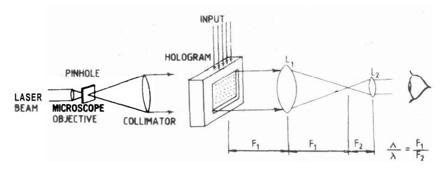
Figure 5. Holographic sonar system.
