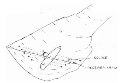
Figure 3. Holographic concept for harbor surveillance.
