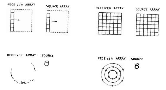
Figure 1. Source and receiver transducer array
