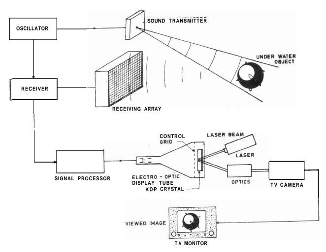
Figure 4. Underwater medium-range holographic system.
