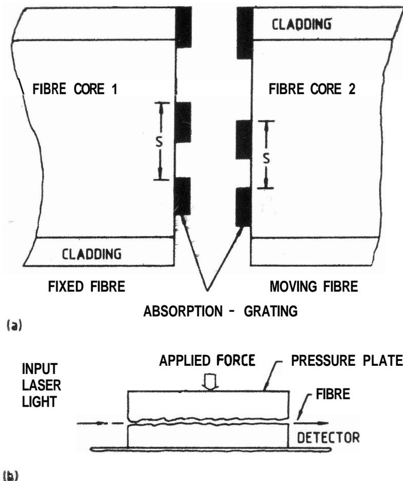
Figure 3. (a) Absorption grating, (b) Microbend hydrophone.
