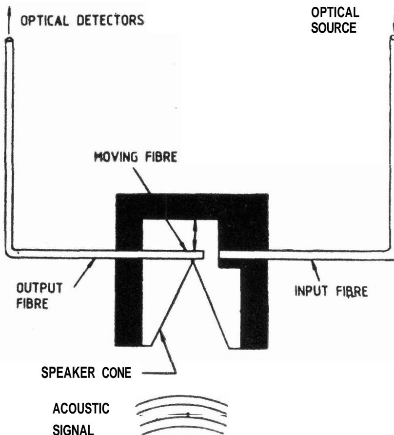
Figure 2. Multimode acoustic hydrophone.
