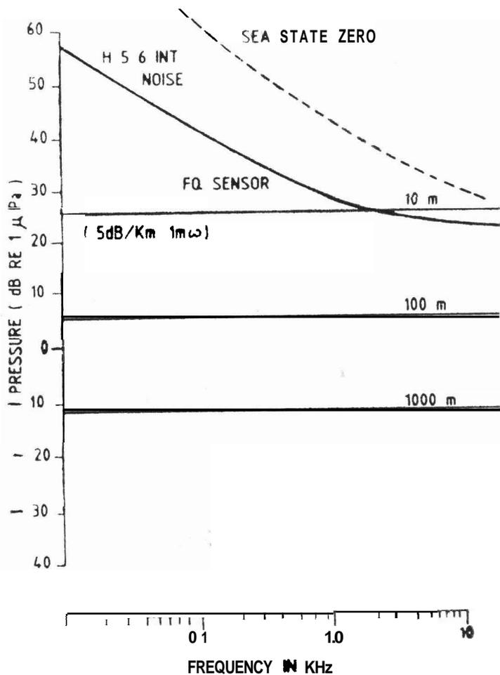
Figure 7. Quantum limited minimum detectable pressures.
