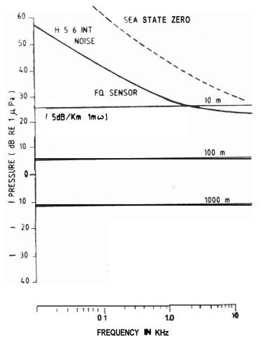
Figure 7. Quantum limited minimum delectable pressures.
