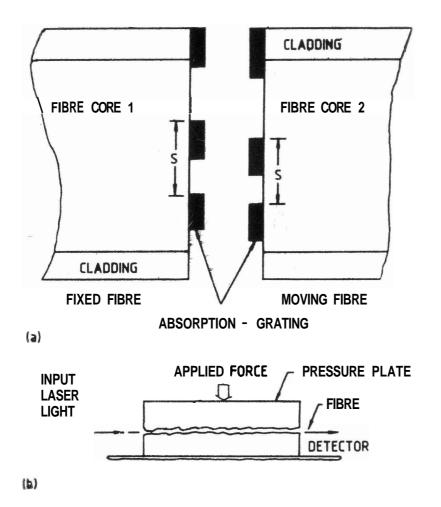
Figure 3. (a) Absorption grating, (b) Microbend hydrophone.
