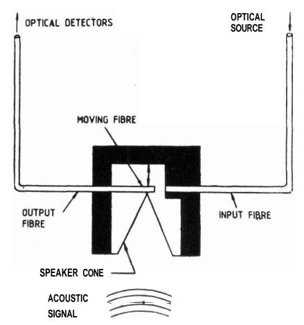
Figure 2. Multimode acoustic hydrophone.
