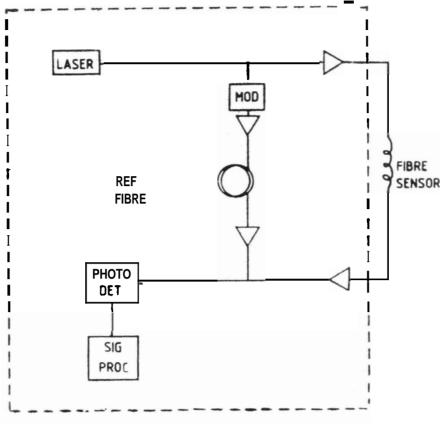
Figure 6. Fibre optic hydrophone.
