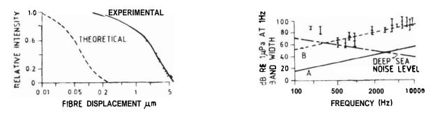
Figure 5. FT1R hydrophone minimum detectable pressure vs frequency theoretical (A) and experimental (B) sensitivity.
