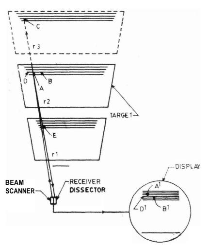
Figure 4. Target discrimination in Synchronous laser television
