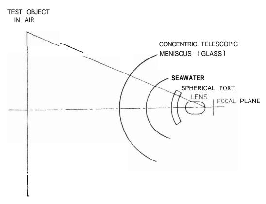
Figure 5. Port hole for underwater camera,
