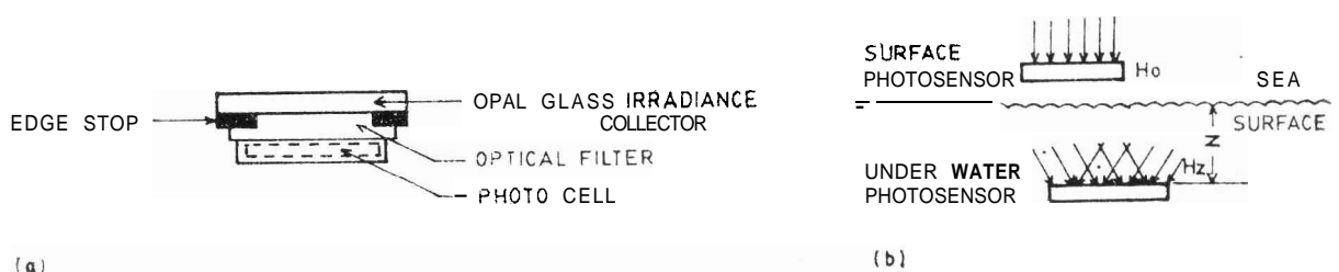
Figure 2. (a) Irradiance collector (b) Measurement of diffuse attenuation coefficient K
