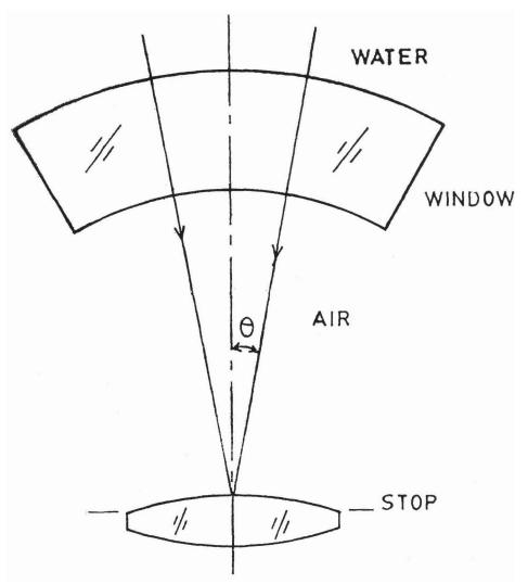
Figure 2. Concentric optical window.
