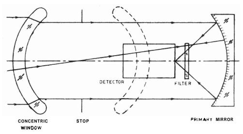
Figure 3. Receiver optics configuration (for low speeds)
