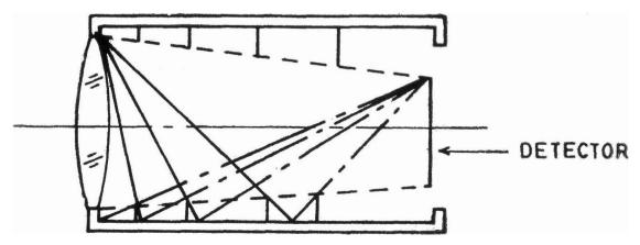
Figure 1. Straylight elimination by baffles.
