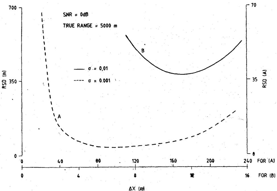
Figure 7. Dependence of range standard deviation on sensor separation distance: non-ideal medium.
