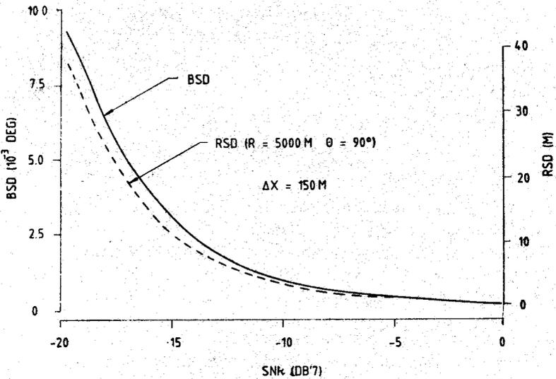
Figure 3. SNR dependence of range and bearing standard deviations : ideal medium.
