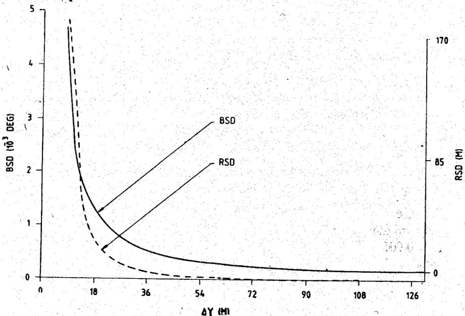
Figure 4. Dependence of range and bearing standard deviations on sensor separation distance : ideal medium.
