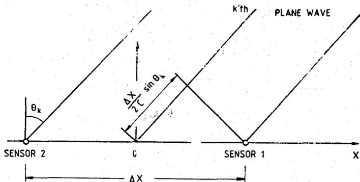
Figure 1. The array geometry for time-delay-estimation.
