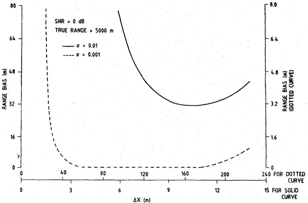
Figure 8. Dependence of range bias on separation distance.
