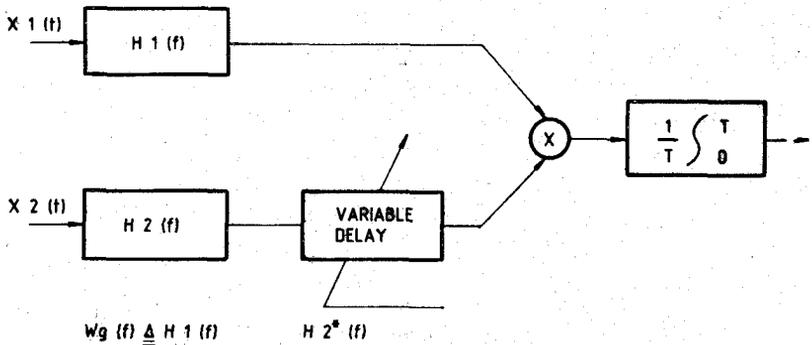
Figure 2. Generalized cross-correlator for time-delay-estimation.
