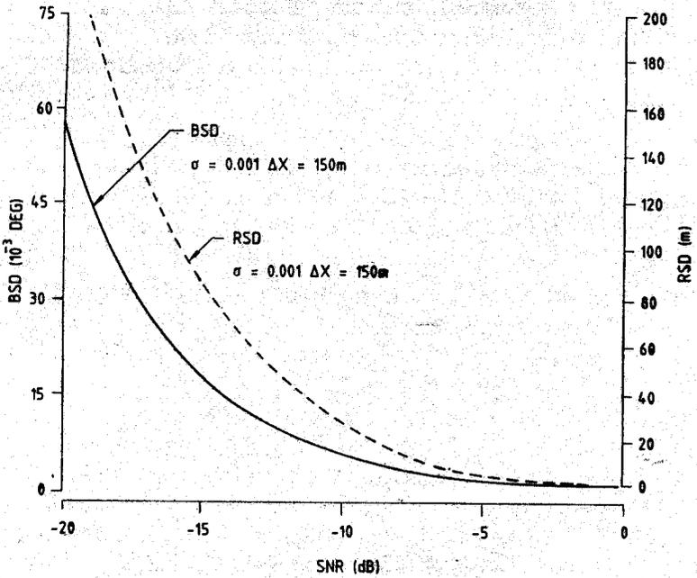
Figure 5. SNR dependence of range and bearing standard deviations : non-ideal medium.
