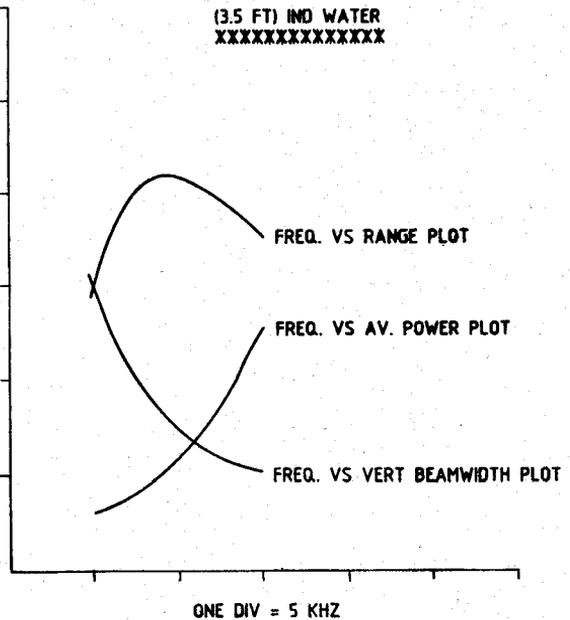
Figure 4. Range, Vert. beamwidth Vs frequency for various Sonar specifications.
