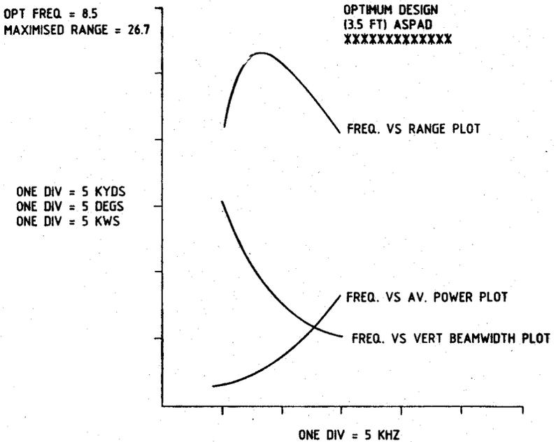
Figure 5. Range, Vert. beamwidth and power Vs frequency for various Sonar specifications.
