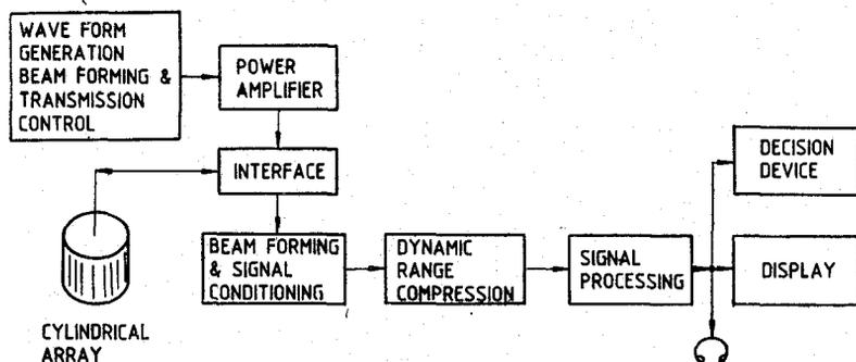
Figure 2. Block schematic of a basic sonar.
