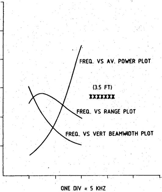
Figure 3. Range, Vert. beamwidth and power Vs frequency for various Sonar specifications.
