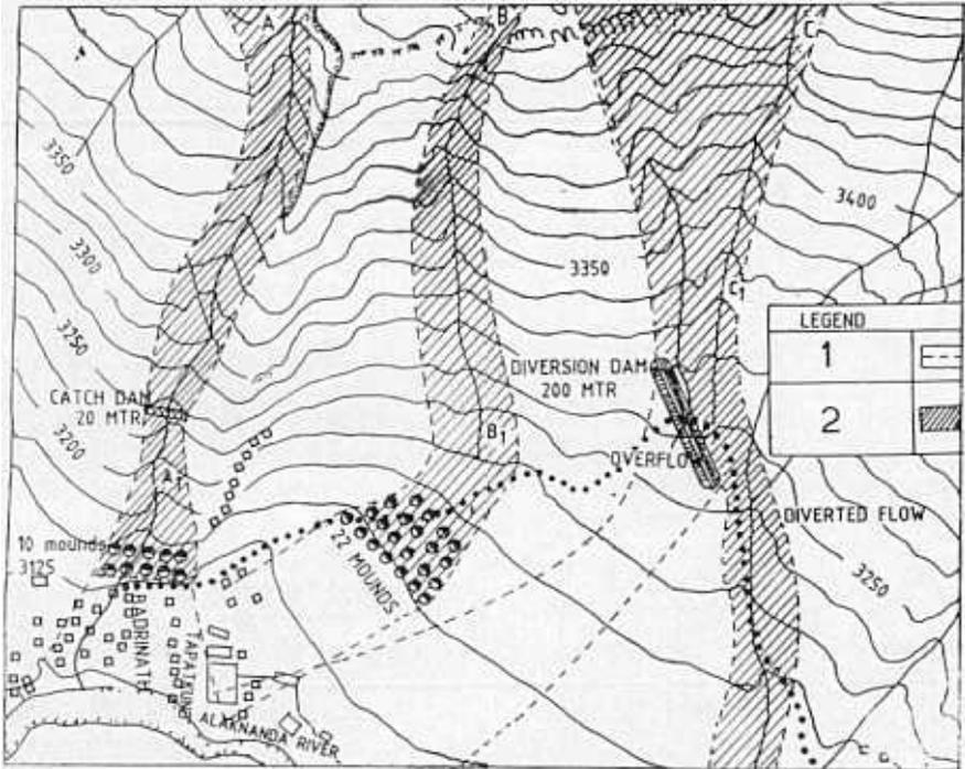
**Figure 6.** Avalanche gullies and the layout of the control structures construction. (Badrinath avalanche area—control interval 25m). Legend 1—Flow boundaries before control structures constructions Legend 2 Avalanche flow with boundaries after control structures construction.
