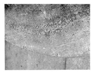
Figure 4. Aluminium bronze propeller blade showing typical cavitation.
