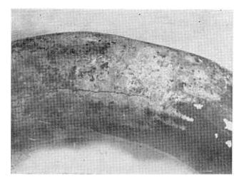
Figure 3. Crack and deposits in a Muntz metal tube.
