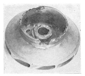
Figure 2. Aluminium impeller failed in service due to galvanic attack.
