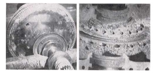
(a) (b) Figure 1 (a & b). Typical chloride pitting of impeller and housing.
