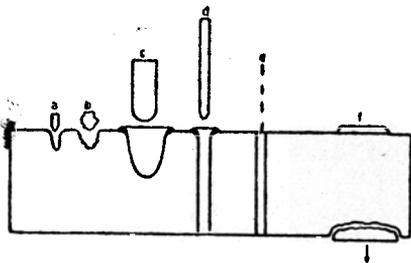
**Figure 1.** Schematic description of damage capabilities of some ammunitions. (a) 7.62 AP shot, (b) missile fragments, (c) 105 APDS shot, (d) 105 FSAPDS penetrator (e) hollow charge, 106 RCL, (f) HESH and (g) pressure pulse from mine.
