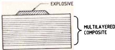
Figure 6. A multilayered composite to subdue shock waves.
