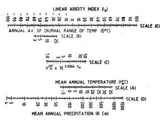
Figure 4. Nomogram for evaluation of linear aridity index  $(I_a)$ . Straight line through scales (A) and (B) gives  $(\sqrt{D} \times 10^{0.0244t}m)$  on scale (C). Straight line through this point and scale (D) gives  $I_a$  on scale (E).
