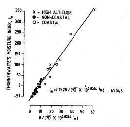
Figure 3. Linear relationship between  $I_m$  and  $R/(\sqrt{D} \times 10^{0.0264t}m)$
