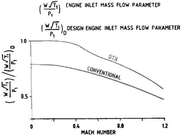
Figure 5. Estimated engine performance—ISA + 30°C sea level, max dry.
