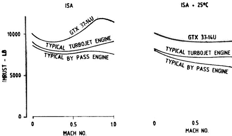
Figure 8. Comparative engine performance—sea level, max dry rating.
