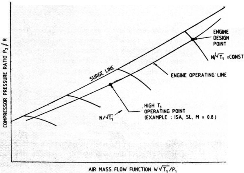
Figure 2. Compressor characteristics.
