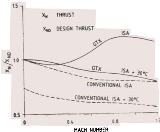
Figure 3. Estimated engine performance—sea level, max dry.
