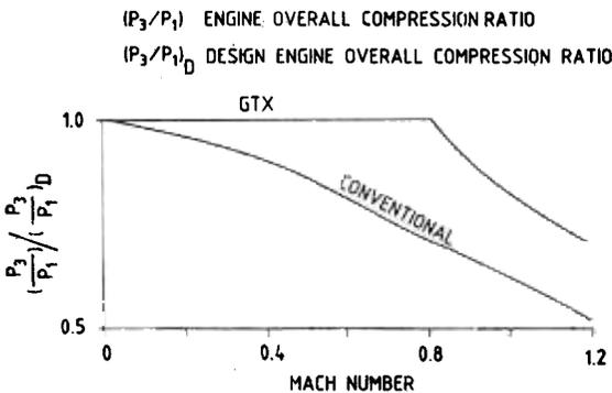
Figure 6. Estimated engine performance—ISA sea level, max dry.
