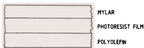
Figure 4. Dry-film photoresist composition.
