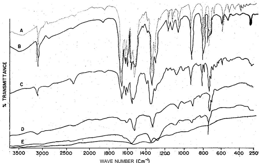
Figure 7. IR spectra of silver 2,4,6-trinitrobenzoate at (A) room temperature, (B) 100°C, (C) 140°C, (D) 150°C, (E) 190°C and (F) 200°C.
