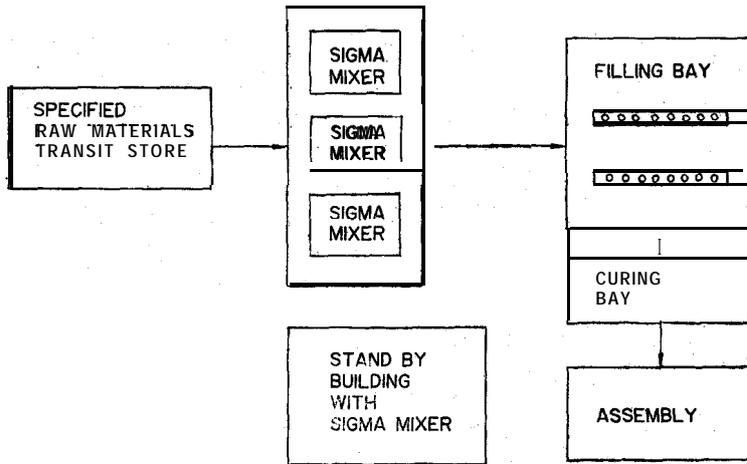
**Figure 5.** Proposed layout of the futuristic processing plant for manufacture of **castable** screening smoke ammunition.
