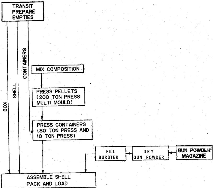
Figure 3. Process description for pelleting method, with conventional screening smoke composition.
