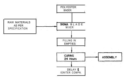
Figure 4. Process description for preparation of castable screening smoke composition.
