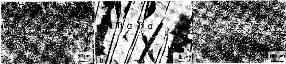
Figure 12. Typical microstructures of different grades of titanium alloys: (a) Cast structure of a near alpha titanium alloy ( Ti-11 ), (b) Retained beta phase present between alpha platelets in an alpha-beta titanium alloys ( VT-9 ), and (c) Alpha precipitation in retained beta grains in a beta titanium alloy ( Beta C ).
