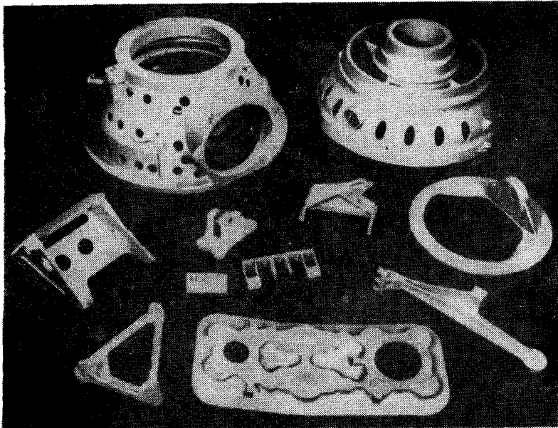
Figure 3. (b) Typical applications of titanium castings : Complex precision castings for aerospace applications.
