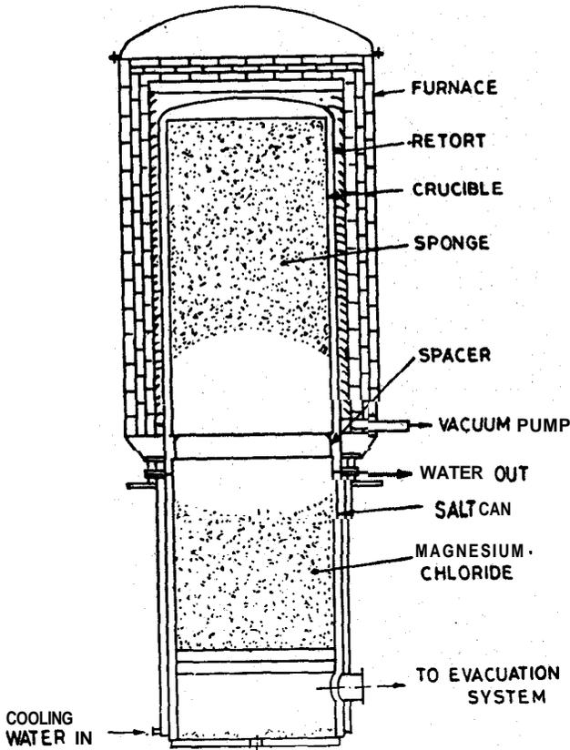
**Figure 9.** Vacuum distillation assembly.
