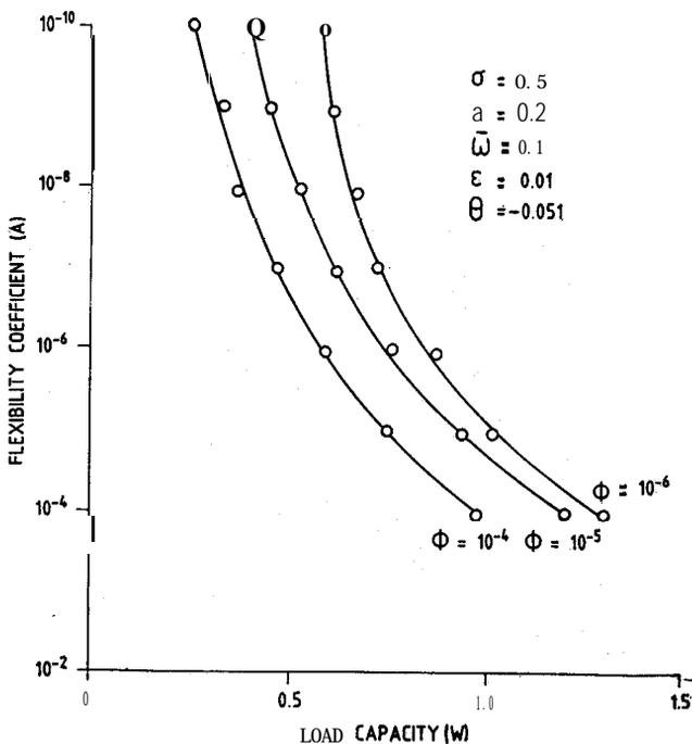
Figure 2. Variation of load capacity  $W$  with flexibility coefficient  $A$  &  $\phi$ .
