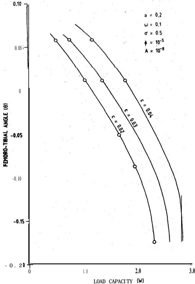
Figure 3. Variation of load capacity with  $\theta$  &  $\epsilon$ .
