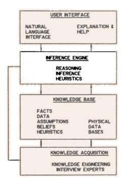
Figure 1. Structure of an expert system.
