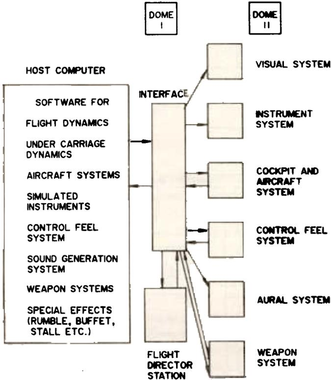
Figure 4. Flight simulation facility PH II.
