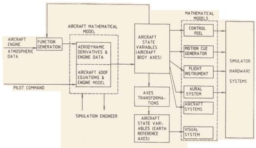
Figure 2. Flight software organization-block diagram.
