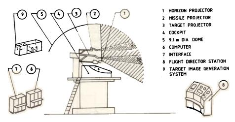
Figure 5. Proposed air combat simulation facility.
