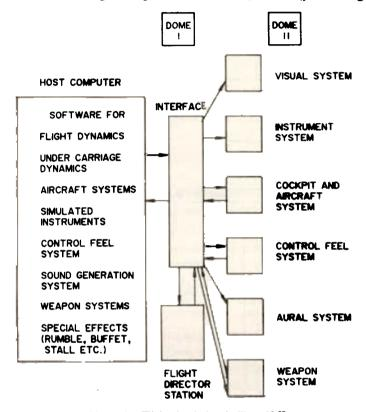
Figure 4. Flight simulation facility PH II.
