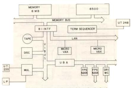
Figure 6. Computer configuration (Air combat simulator)
