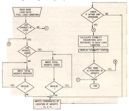
Figure 4. Ship loading alternations.
