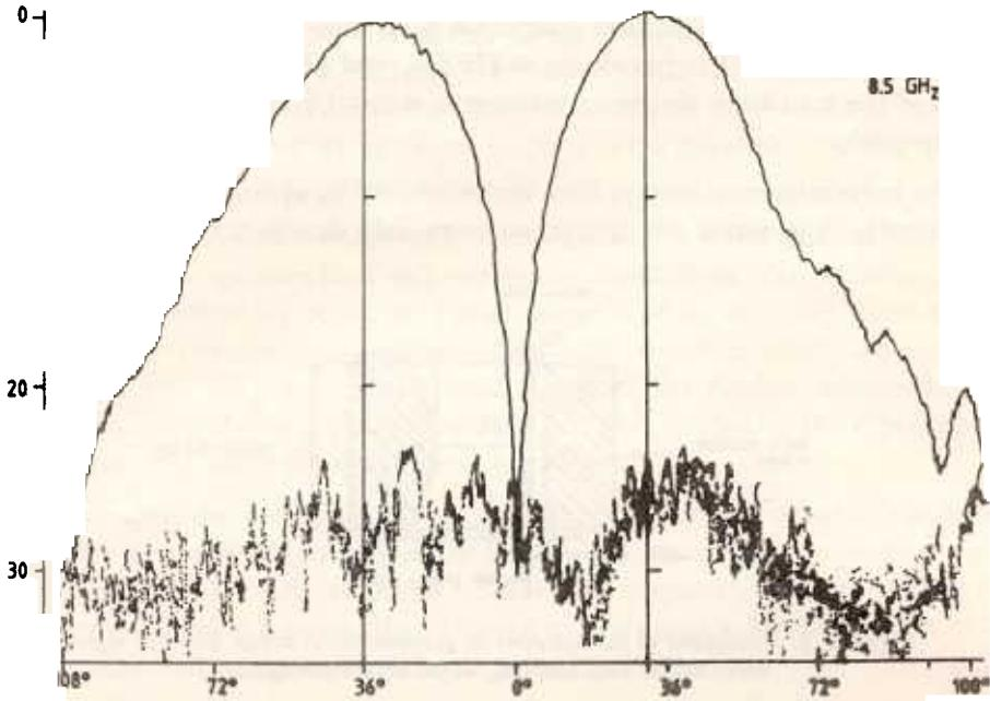
Figure 4(a) E plane and its cross-polarised radiation patterns of the antenna at frequency in 8.5 GHz band.
