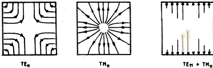
Figure 2. Aperture field distribution of higher order modes  $TE_{11}$ ,  $TM_{11}$  and  $TE_{11} + TM_{11}$  in a square waveguide.
