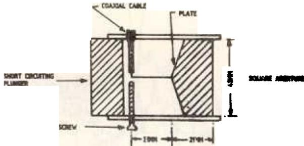
Figure 3. Schematic of the assembly to generate the resultant effect of higher order modes  $TE_{11}$  and  $TM_{11}$  in the square waveguide
