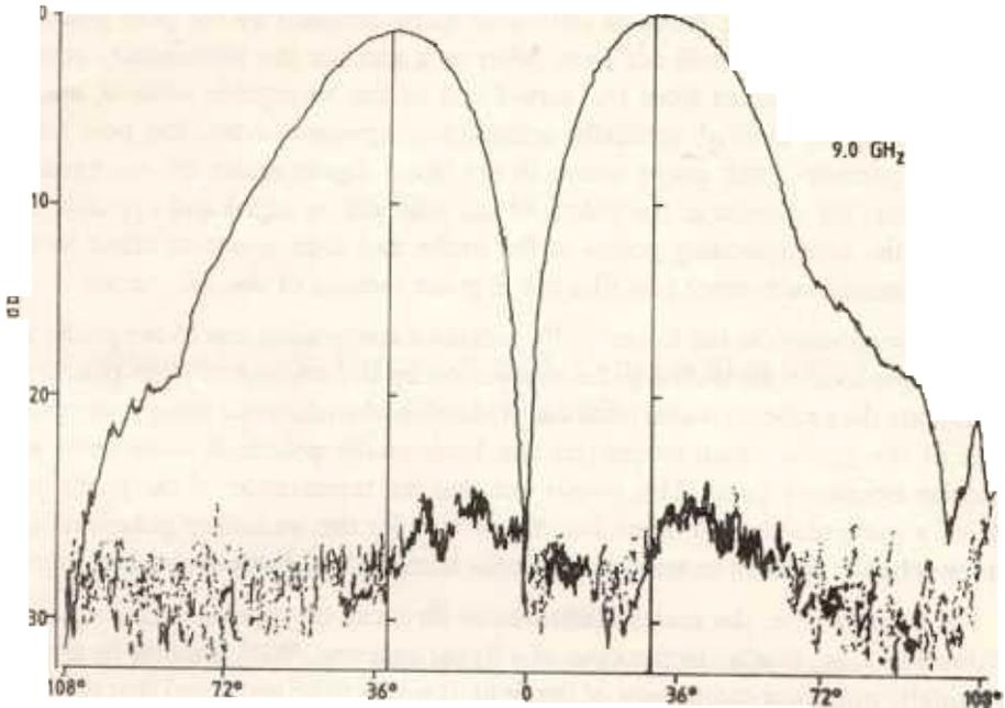
Figure 4(c) E plane and its cross-polarised radiation patterns of the antenna at frequency in 9.0 GHz band.
