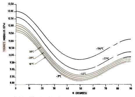
Figure 1. Variation of Young's modulus of ice with angle of orientation between c-axis and direction of measurement.
