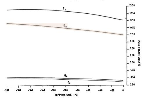
Figure 3. Variation of Young's and shear moduli parallel to  $(E_c, G_c)$ , and normal to  $(E_s, G_s)$  the c-axis, with temperature.
