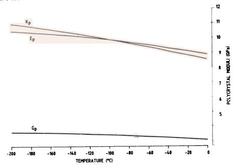
Figure 5. Variation of the shear  $(G_p)$ , bulk  $(K_p)$  and Young's  $(E_p)$  moduli for polycrystalline ice, with temperature.
