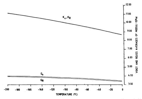
Figure 4. Variation of the Voigt and Reuss averages of shear  $(G_v, G_r)$  and bulk  $(K_v, K_r)$  moduli with temperature.
