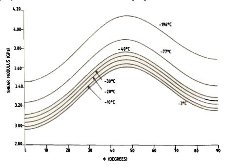
Figure 2. Variation of shear or rigidity modulus with angle of orientation.
